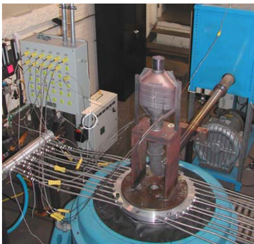
Figure 21: Hot-Vibe Test Bench
