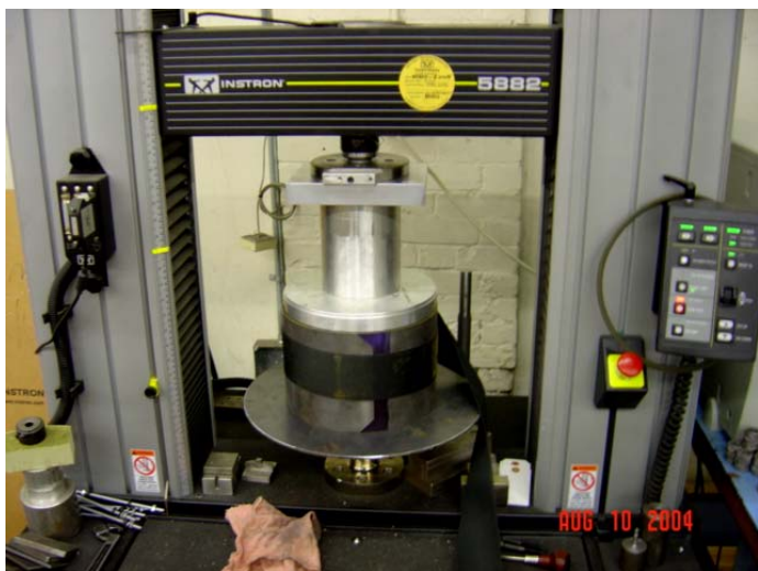
Figure 6: An Instron load frame with a tourniquet style can mock-up.
