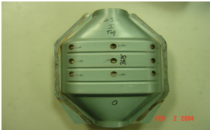
Figure 23: Gap Checking with Drilled Holes
