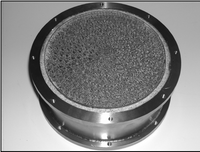
Figure 21: Wiremesh substrate in single seam converter assembly
